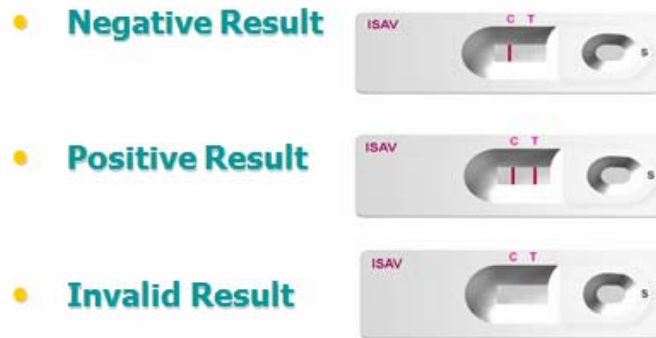
Figure 2.1.2. An immunochromatography kit showing negative, positive and invalid results.
